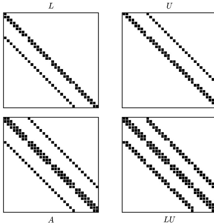
**Figure 10.2** The ILU(0) factorization for a five-point matrix.
