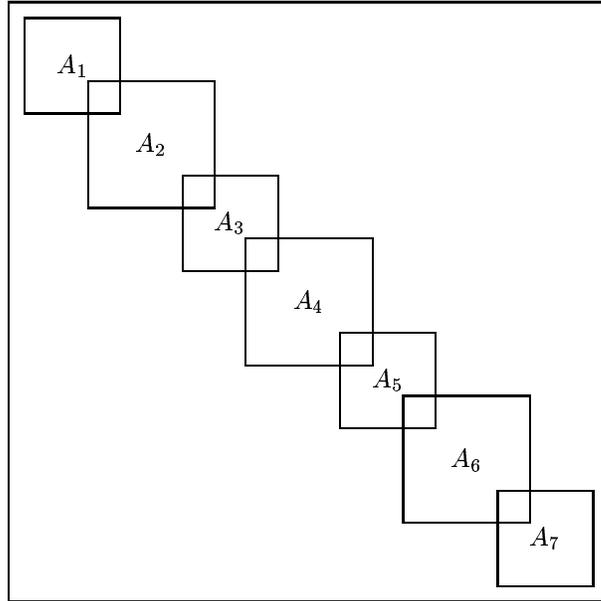
**Figure 12.1** *The block-Jacobi matrix with overlapping blocks.*
