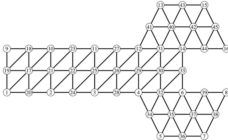
**Figure 3.1** A finite element grid model.
