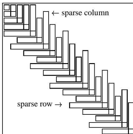
**Figure 10.13** Illustration of the sparse skyline format.
